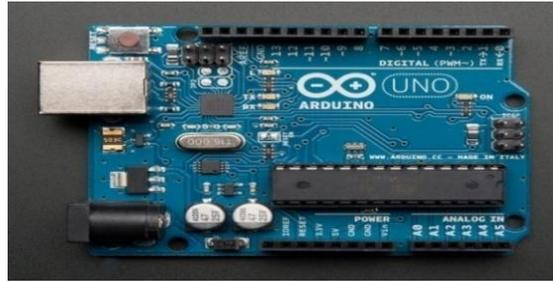
**Fig-5: arduino board**
