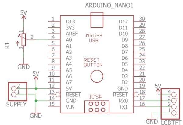
Fig. 3. Height detector circuit
