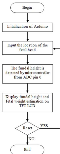
Fig. 2. The Flowchart of the Arduino Program
