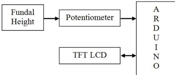
Fig. 1. The diagram block of the Modul
