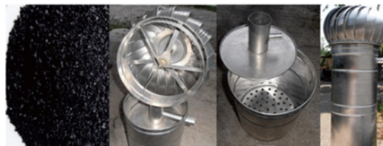
Figure 1. Active Carbon and Cyclone Ventilator Modification
